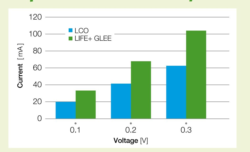
Out-of-plane conductivity analysis shows an increse in electrical conductivity of the electrode containing Cu-coated particles. Calculated resistance values are of  $2.9 \Omega$  and  $4.81 \Omega$ .
