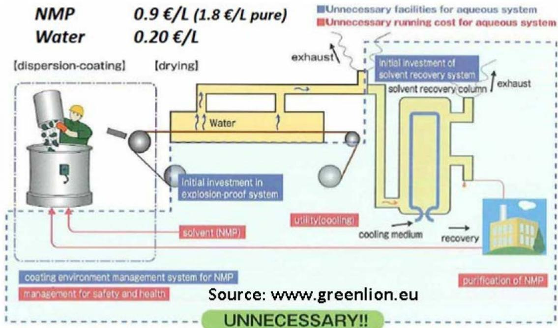
Fig. 4: additional costs for cathode production that become unnecessary by using THE LIFE+GLEE aqueous based process.
